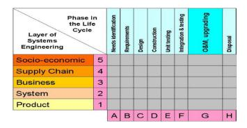
**Figure 1.** The HKM Framework for understanding systems engineering. [Color figure can be viewed in the online issue, which is available at wileyonlinelibrary.com.]
